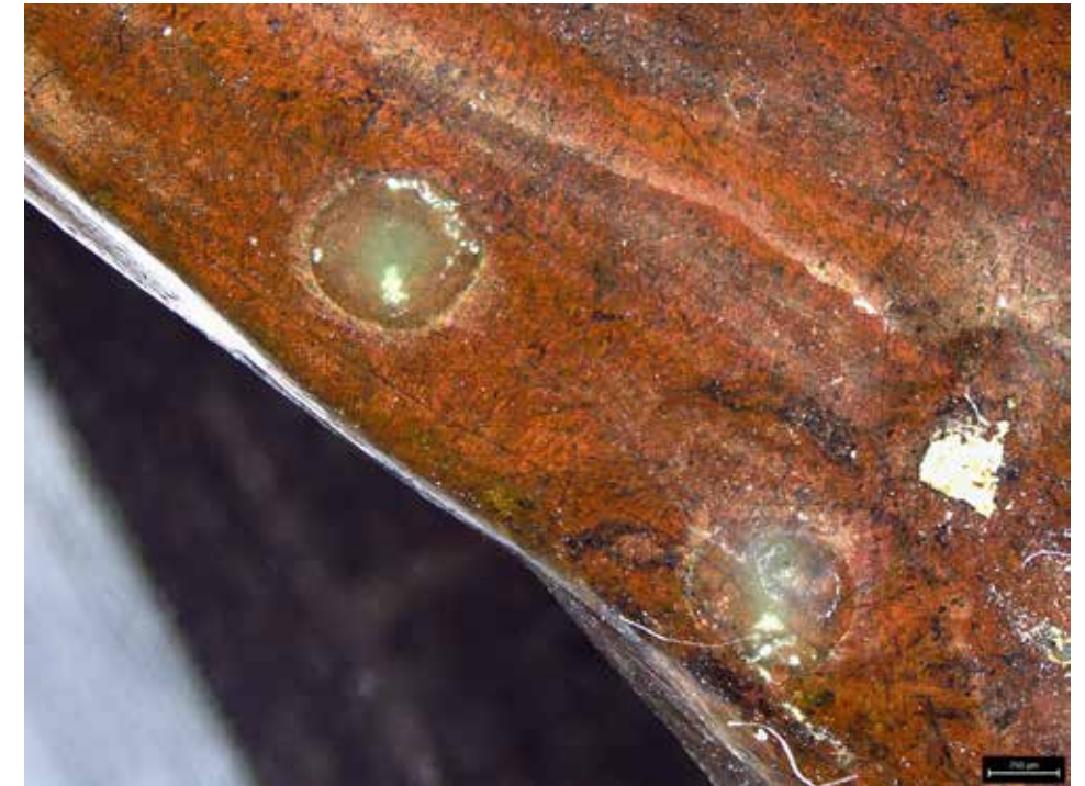
Fig. 17. Digital image of patina with remains of wax and gesso in the arm of the Bronze Crucified Christ , IOMR Collection
