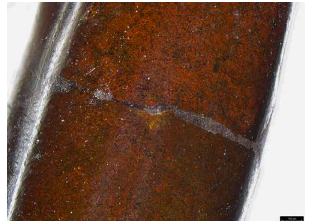
Fig. 18. Image silver soft solder in the arm of the Bronze Crucified Christ , IOMR Collection
